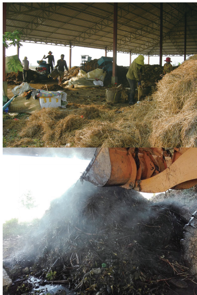
Figure 12: Windrow Composting of Organic Waste
