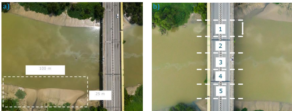
Figure 17. Visual counting methods from a riverbank (a) and bridge (b). Source: van Emmerik, 2020.
