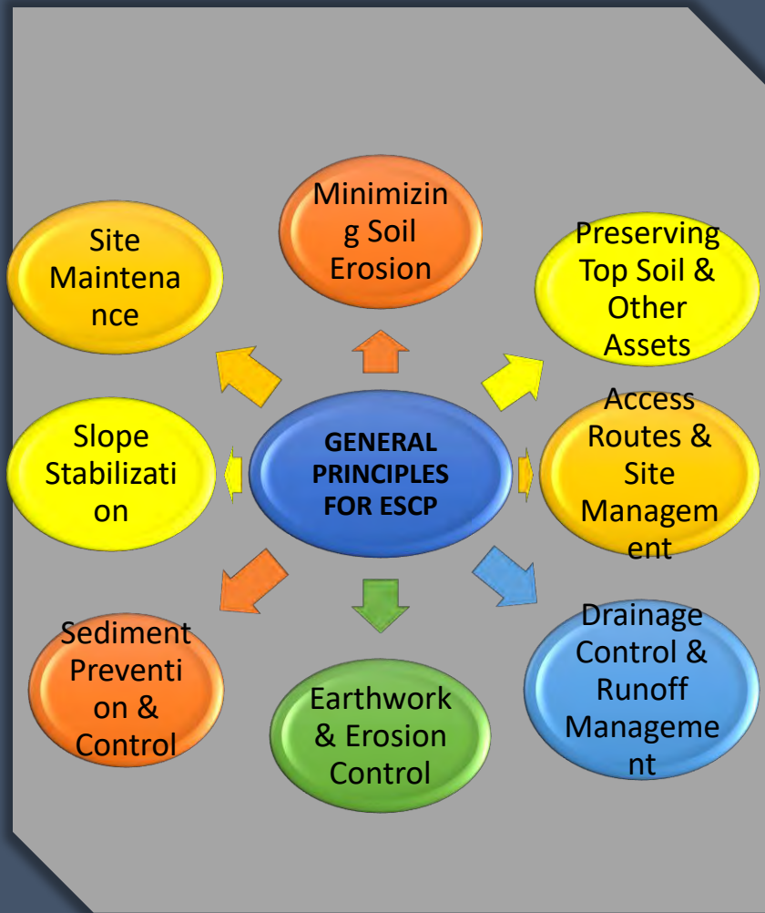
Erosion and Sediment Control Principles
