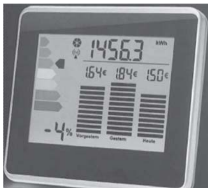
Energy Usage Monitor and Sensors(eQ-3)
