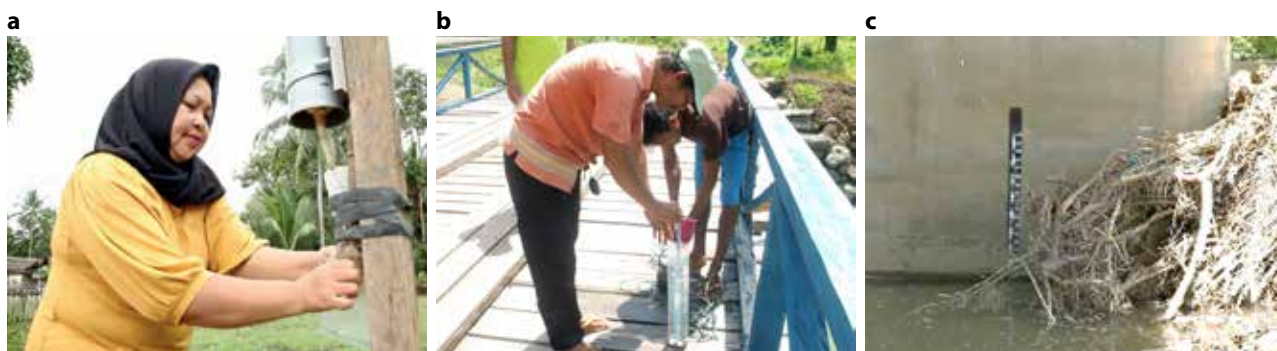
Figure 8. a) Rainfall measurement, b) turbidity measurement, c) water height measurement
