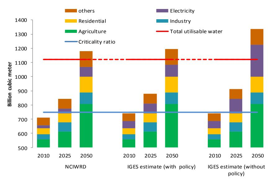
Note: Estimated water demand with policy intervention basically considers the closed loop wet cooling system installed after June 1999 and without policy water demand is a reference estimate of continuation of use of open loop wet cooling system.
