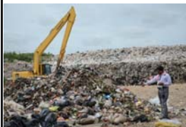
Homogenizing and forming the pile
