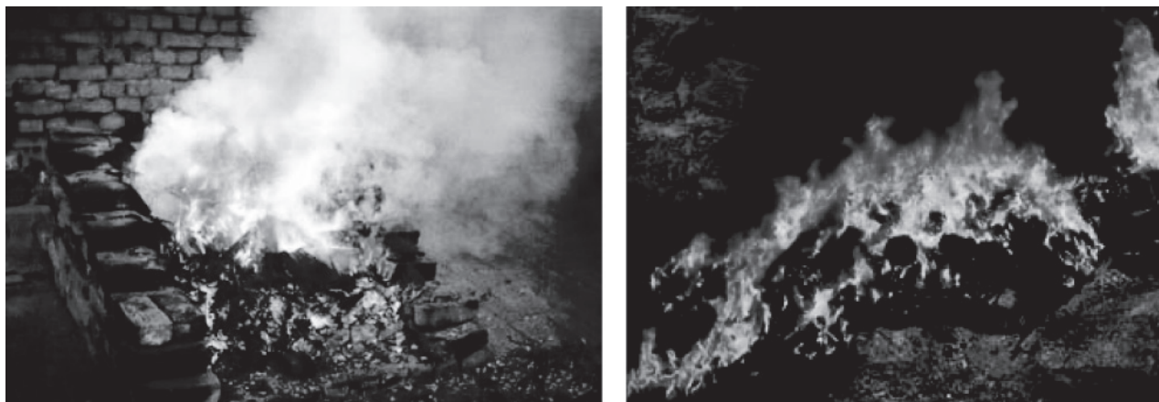
Figure 4: Burning of WEEE to Recover Precious Metals
