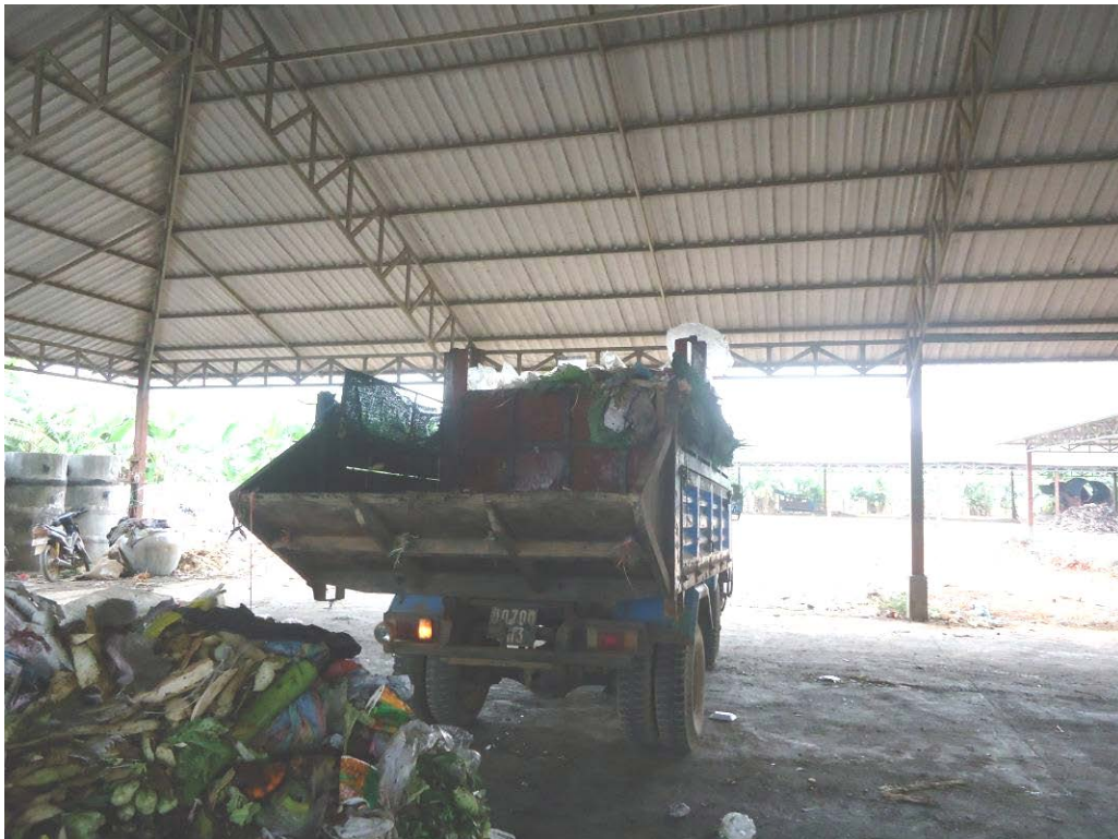
Figure 17: Truck of Phsar Boeng Chhouk with two chambers for loading separated waste
