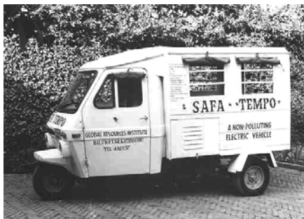
Figure B.1 A typical battery-operated three-wheeler in Kathmandu Valley
