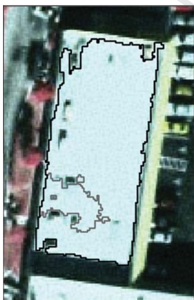
Fig. 1. Segment generated at a fine scale (border shown as a grey line) located within a segment generated at a coarser scale (border shown as a black line).
