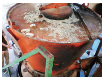
Fig.3 Use of crop residues for electricity generation
