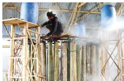
The current bamboo treatment system in operation – each bamboo is stacked vertically and filled with a treatment solution while being smoked
